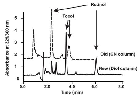
Figure 1. Since it was not possible to find an exact replacement for the NH2 guard column in the former method, we replaced the CN analytical column with a Diol column resulting in a reversal of the peak elution
